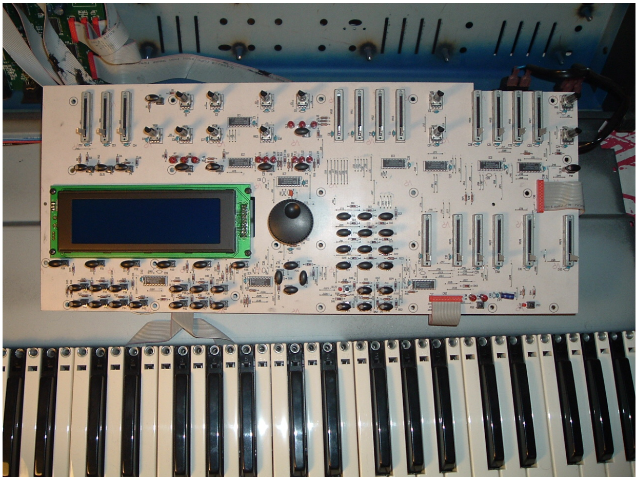
Fig 4: Interior of OB-12, shown with top panel PCB resting freely on bottom panel.
