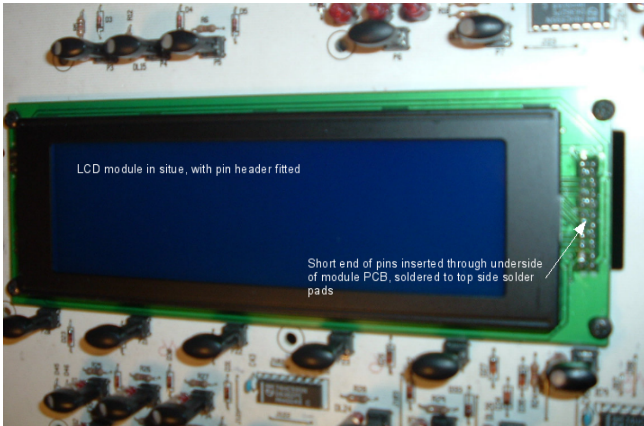
Fig 1: LCD module showing header pin soldering
