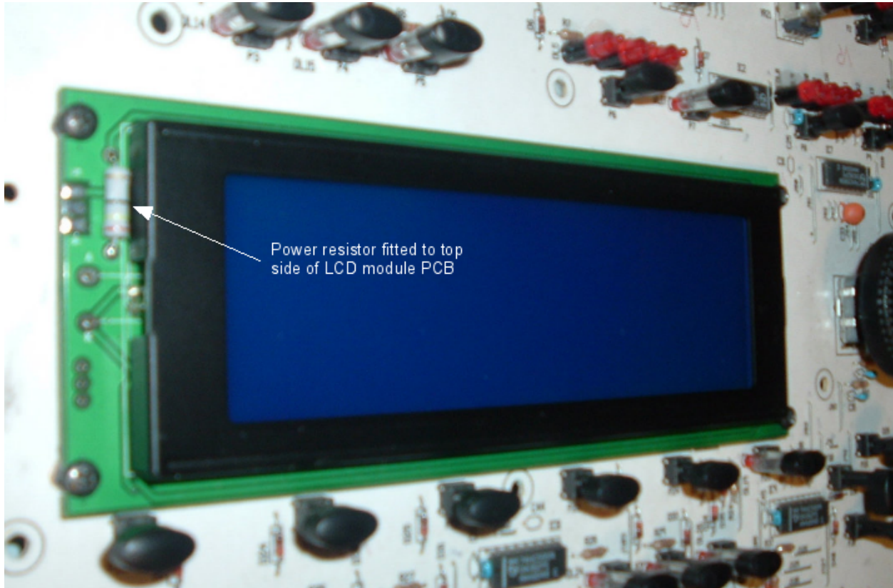
Fig 2: LCD module showing power resistor fitted to top side of PCB
